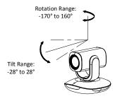
Figure 2-3 Angle Adjustment
